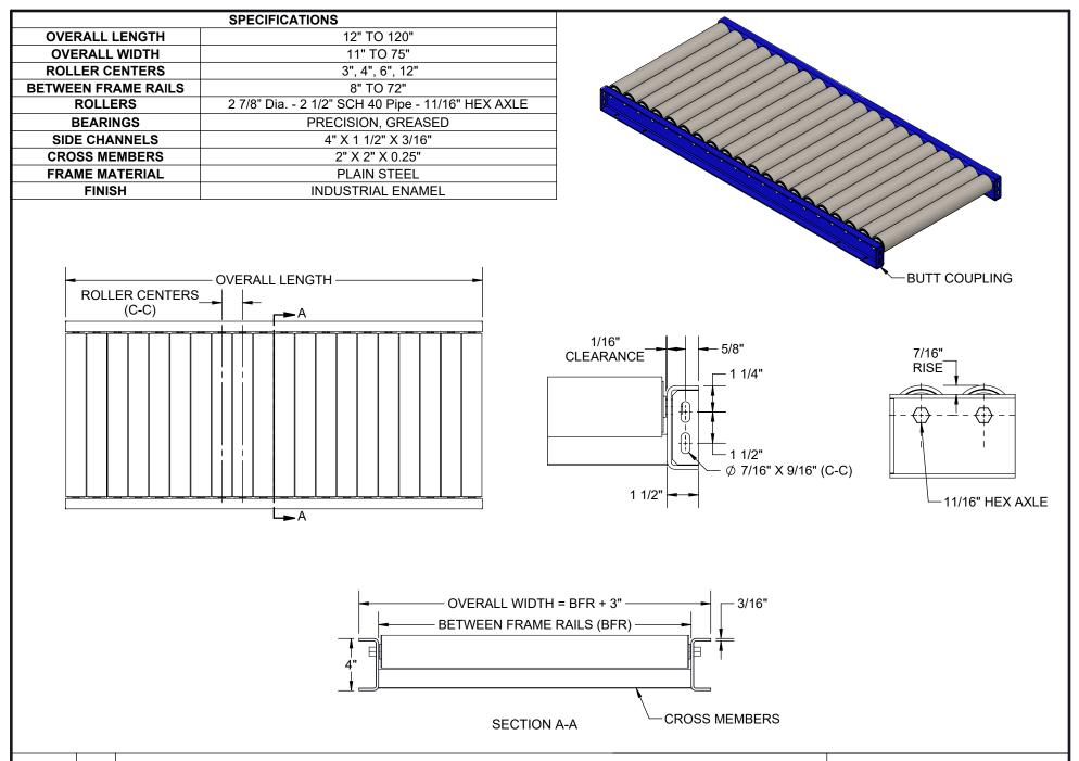
Model: GR – 2925 Gravity Roller Conveyor
