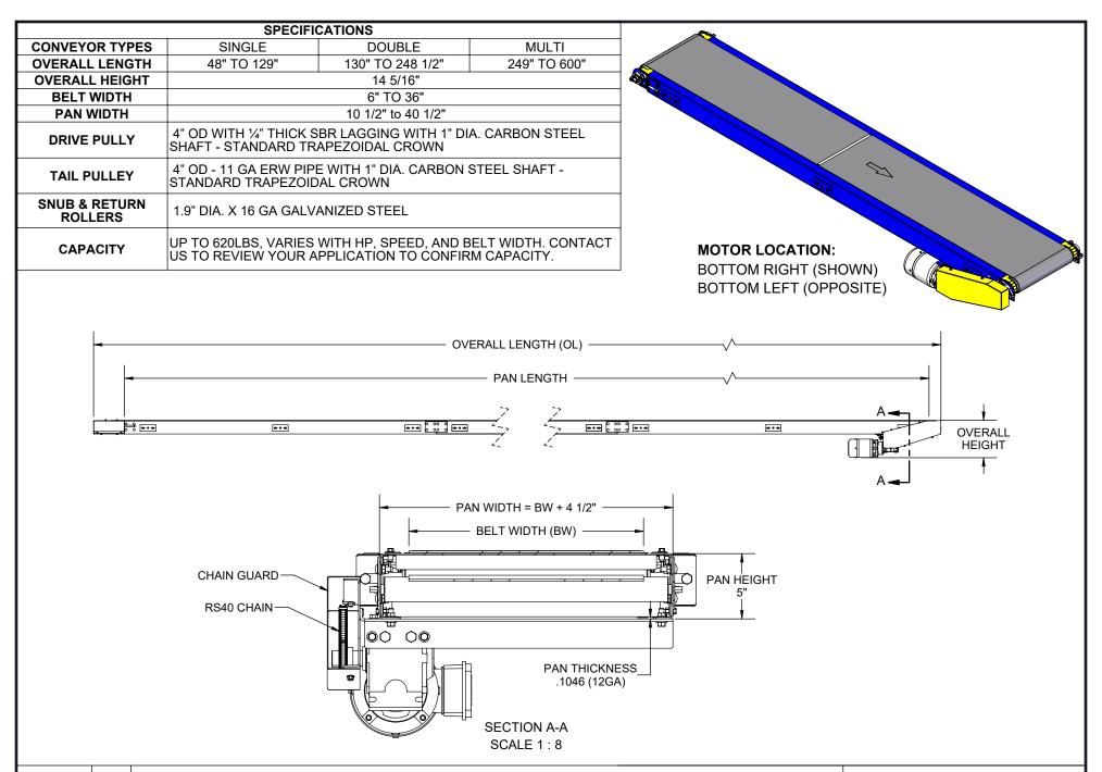
Model: MDSB – Medium Duty Slider Bed Belt Conveyor
