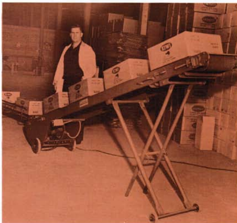
ABOVE: A Rolift Jr. lifts cartons for warehousing in the plant of Langley, Harris Co. Ltd., Toronto, Ont. Attached to a gravity conveyor, it performs many tasks.
