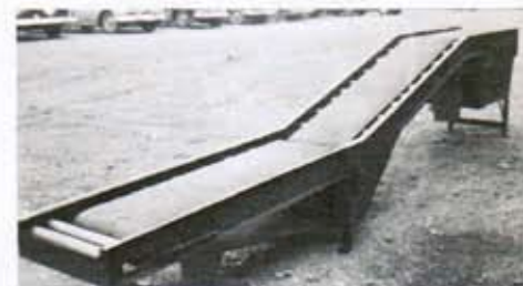
Special Heavy Duty Loading Dock Conveyor can handle live loads of over 500 pounds.
