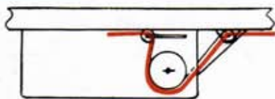
Diagram (F) Shows the Rolmaster "S-Drive" arrangement. This permits easily adjustable belt take-up by movement of snub roll over drive pulley. Adjustment is very easy as all adjusting nuts are on outside of drive; take-up is approximately 18" of belt and this eliminates excessive wear of belt travelling around two extra rolls as normally used on other equipment. Also because of this arrangement more power is transmitted directly to moving the actual load as there are two less rolls between drive roll and load itself.
