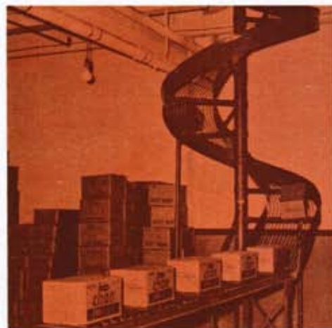
Special Spiral "Slide" Chute built for O'Cedar of Canada Limited. An effective space saving device.
