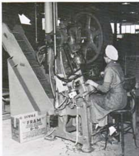
This Punch Press is at Fram Canada Ltd., manufacturers of filters. Note the special Rolmaster Conveyor which carries parts to production line or other stations.
