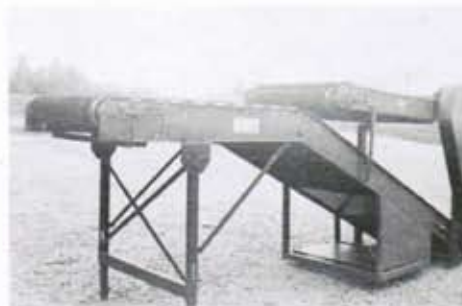
Specially designed Bag Flattener uses Rolmaster Powered Unit to flatten out bags of soft materials, thus saving much space in storing and shipping.
